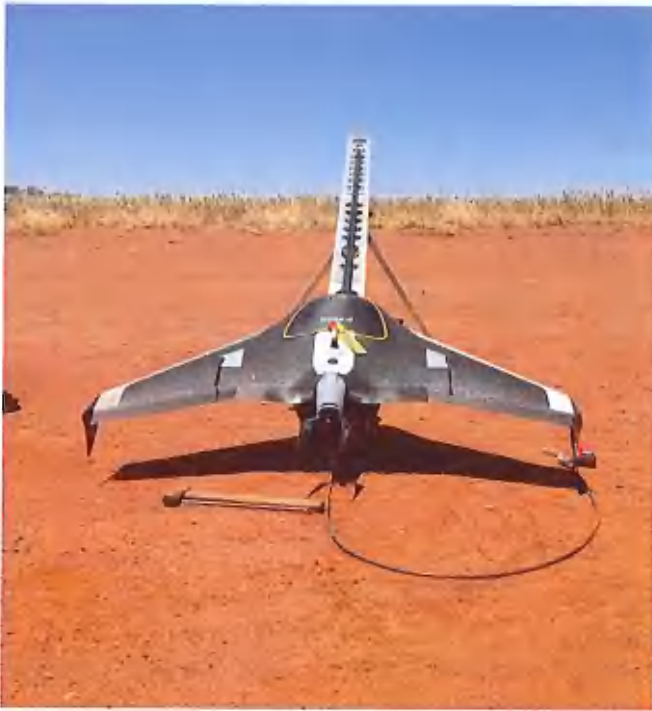
Image 1: UX5 - fixed wing Weight: 2.5 kg Dimensions: 100 x 65 x 10 cm Endurance: 50 min Range: 60 km
