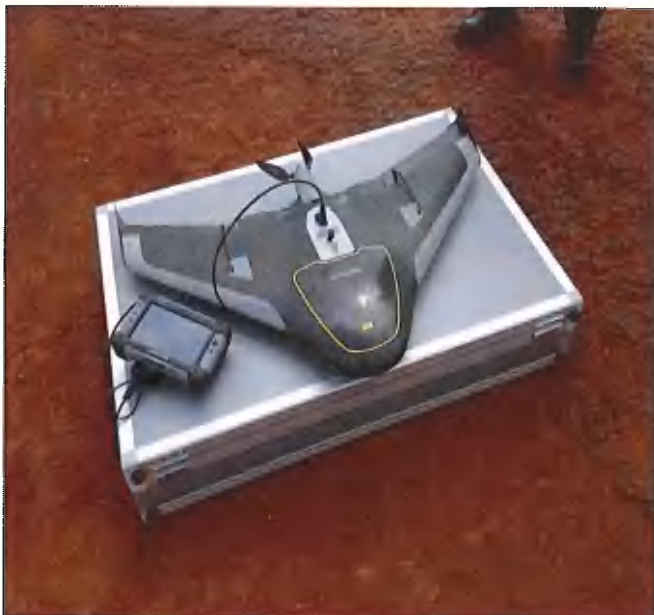
Image 3: eBee – Fixed wings Weight: 0.7kg Dimensions: 910cm wing span Endurance: 45 min Range: 10km 2
