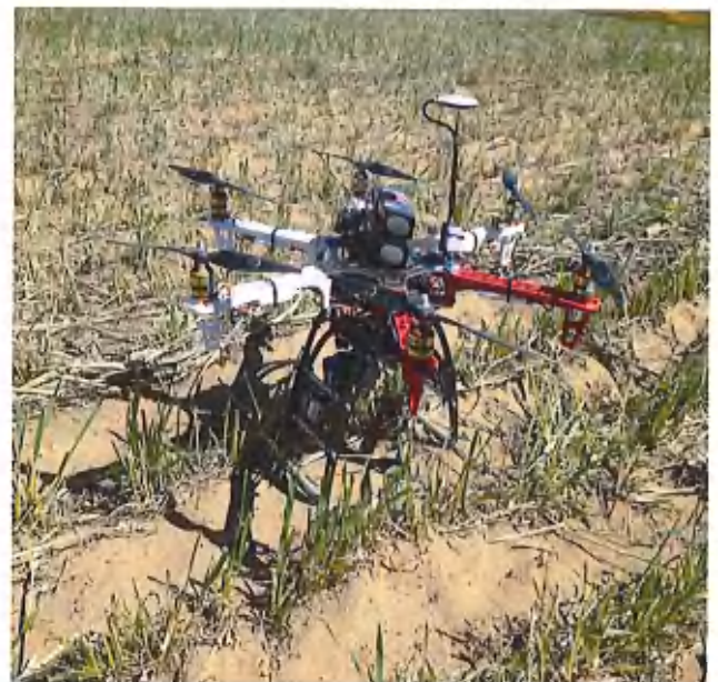
Image 4: F550 – multi copter Weight: 1.8 kg Dimensions: 280 x 320 x 280 mm Endurance: 185 min Range: 6 km 2
