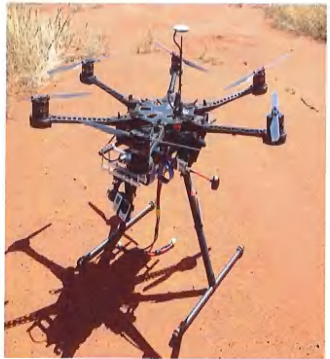
Image 2: S800 – multi copter Weight: 2.6 kg Dimensions: 320 x 800 x 460 mm Endurance: 20 min Range: 20 km
